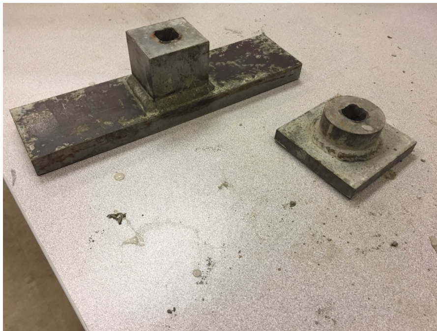
Figure 12. Tamping plate for shrinkage prisms (left) and tamping plate for MOR beams (right).
