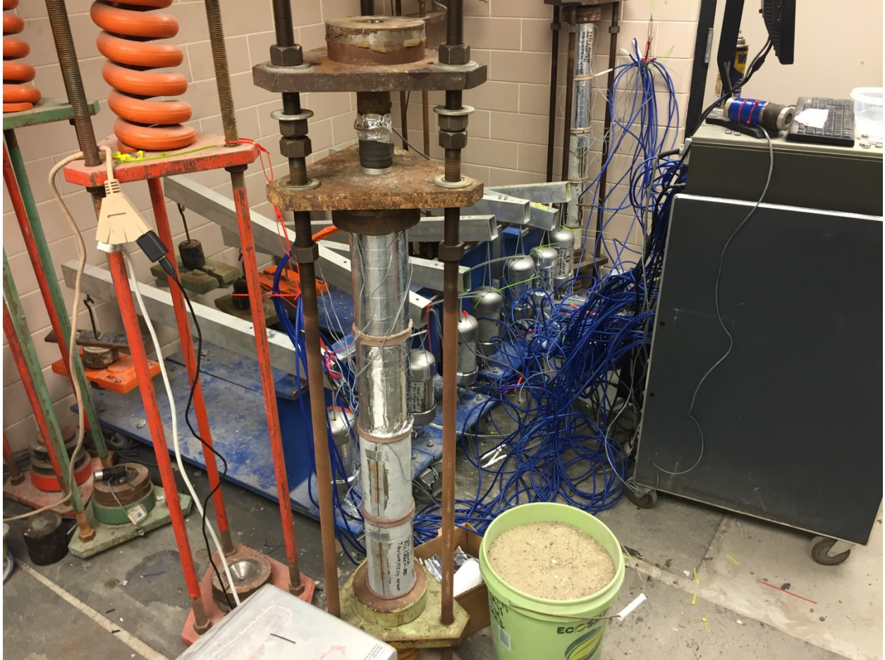
Figure K4. Compressive and Tensile Creep Testing Setup in Environmentally-Controlled Room.
