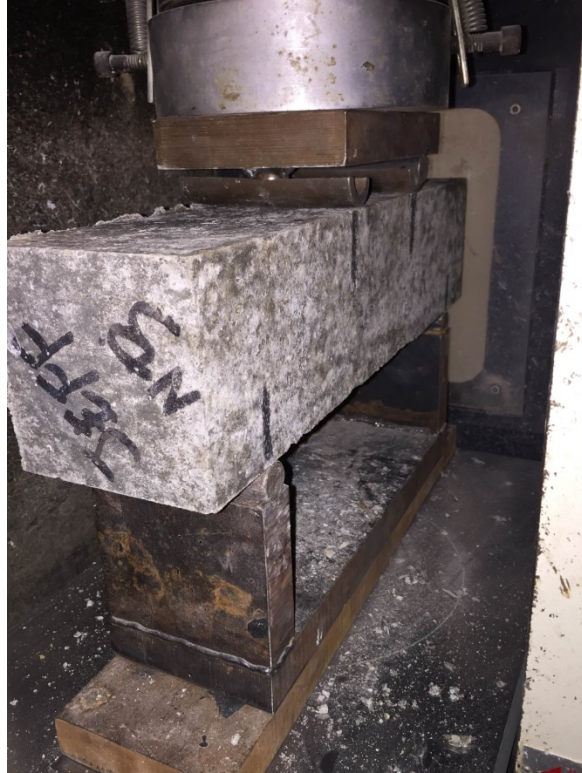
Figure 11. 100x100x400 mm (4x4x16 in) MOR beam specimen being tested in four-point bending.
