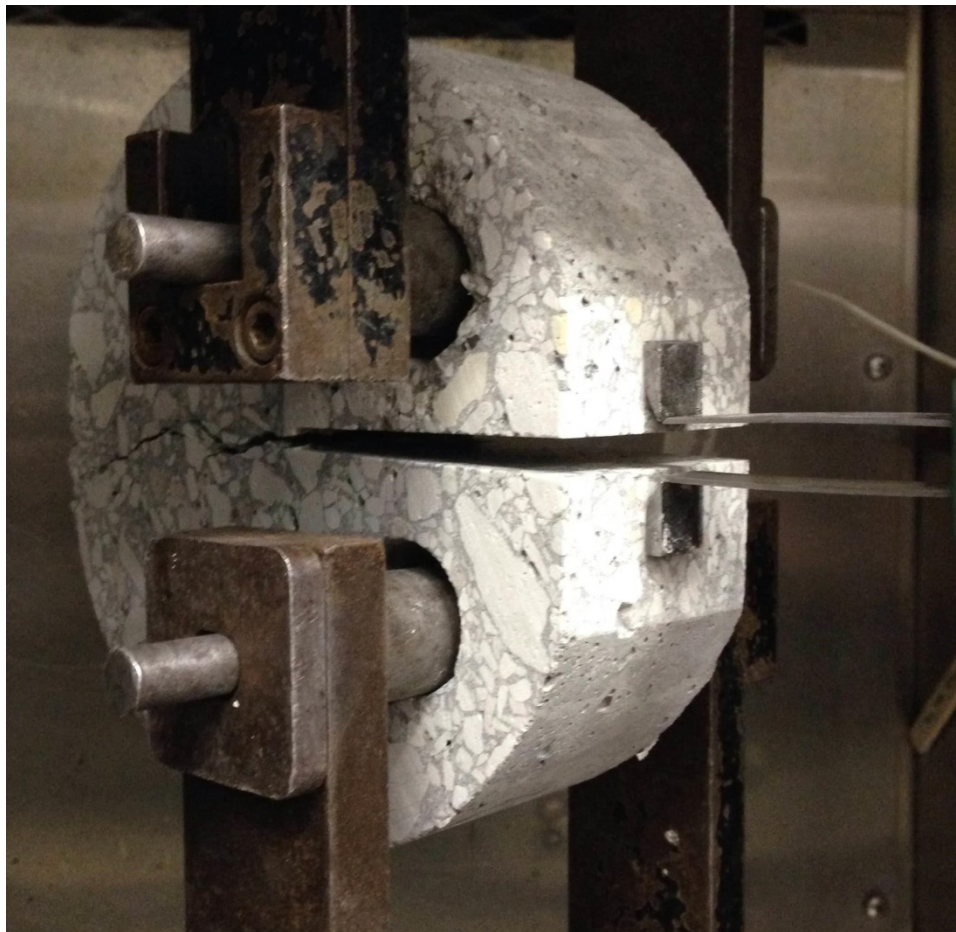
Figure G4. DCT Specimen Loaded in Tension with Clip Gauge (right) Measuring Crack-Mouth Opening Displacement (CMOD).
