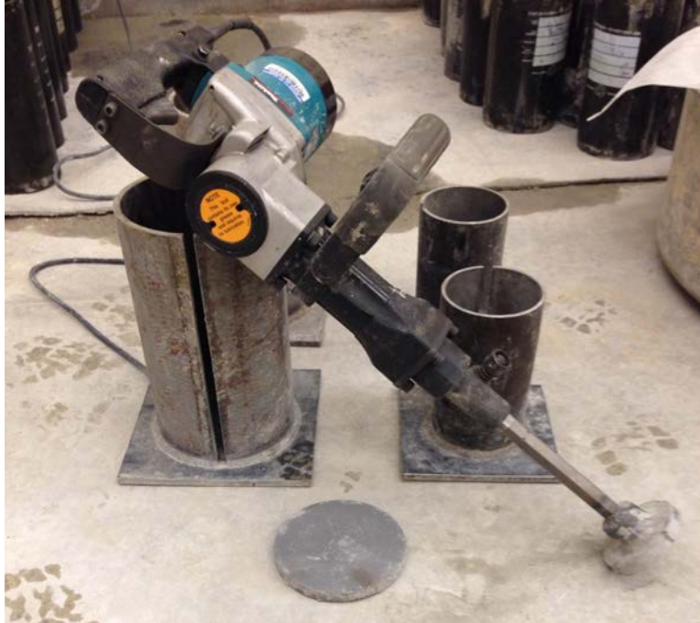
Figure 7. Compaction equipment for RCC cylinders.
