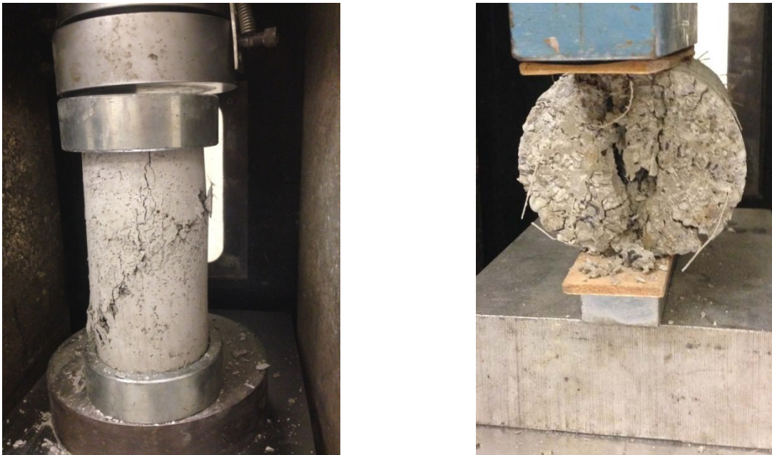
Figure I3. Failure of Unconfined Compressive (left) and Split Tensile Strength (right) Specimens.
