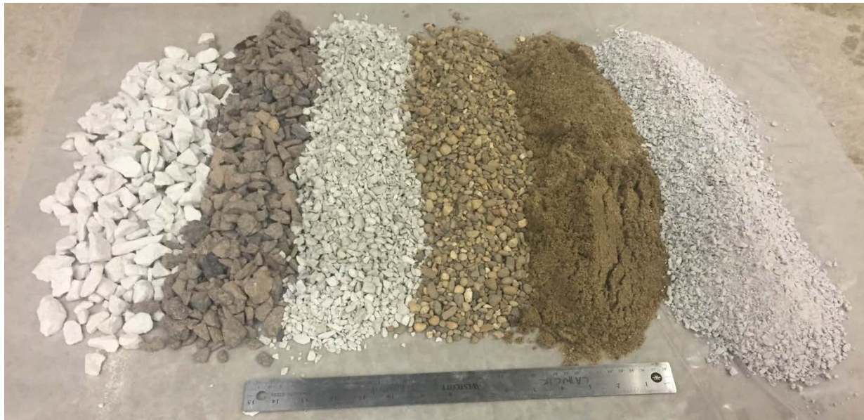
Figure 21. Aggregates used in this Study. From left to right: Coarse Dolomite, Coarse Trap Rock, Intermediate Dolomite, Coarse River Gravel, Natural Sand, and Manufactured Sand.
