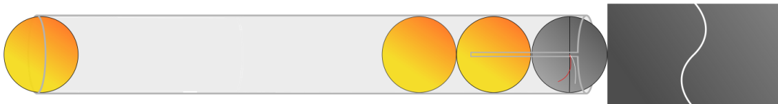
Figure 2.6: Calibration setup. The instrumented bead is placed between two pulse-shaping beads and the Hopkinson bar. Another bead is propelled into the granular chain by a gas gun.
