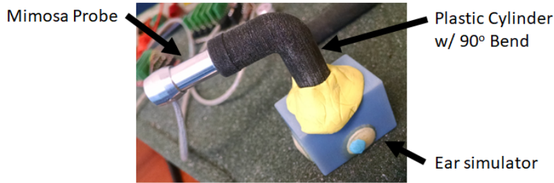
Figure 5.12: Measurement of a 90^\circ bend in a uniform-area horn 7.5 [mm] in diameter.
