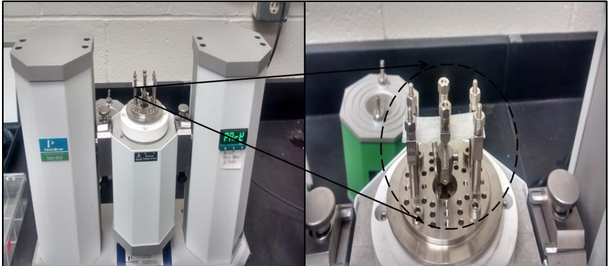
Figure 4.7: DMA Setup (Perkin Elmer DMA 8000)
