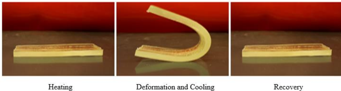
Figure 6.4: SMP specimen undergoing shape memory cycle
