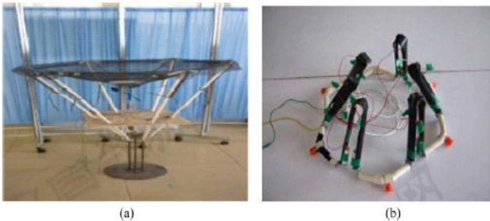
Figure 2.8: The space deployable mesh-surface antenna model: (a) deployed SMPC antenna and (b) packaged SMPC thin shells (Liu et al., 2014)
