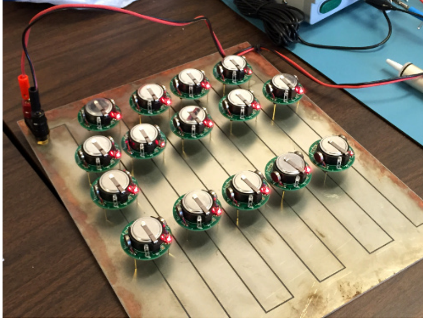
Figure 17: Shinerbots Charging System
