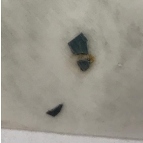
Figure 13. Cracked sample after aggressive lapping
