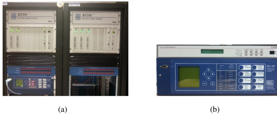
Figure 4.6: (a) RTDS; (b) hardware PMU used for the experiments.
