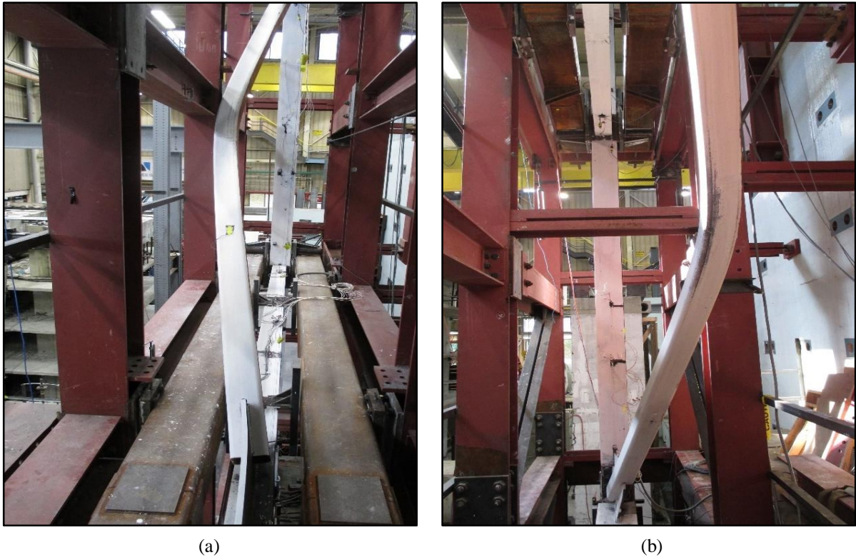
Figure 4.25 – Buckling braces, R = 3.25 split-x OCBF. (a) Story 2 South brace; and (b) Story 1 South brace with hinge region spread over 4 times the brace depth.
