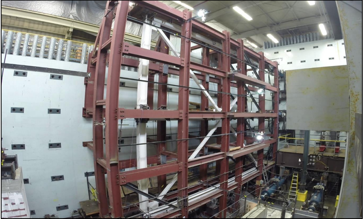
Figure 4.21 – Overview of R = 3.25 split-x OCBF, stabilizing frame, and actuators.
