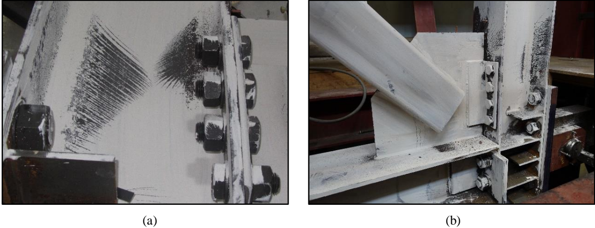
Figure 4.20 – Lower Story 1 column (Level 1) plastic hinging, R = 3 chevron CBF Phase IV: (a) South column; and (b) North column.
