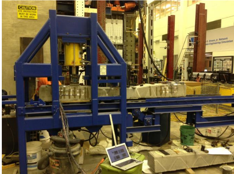
Figure 4.8 Vertical Rail Seat Loading Applied by STT
