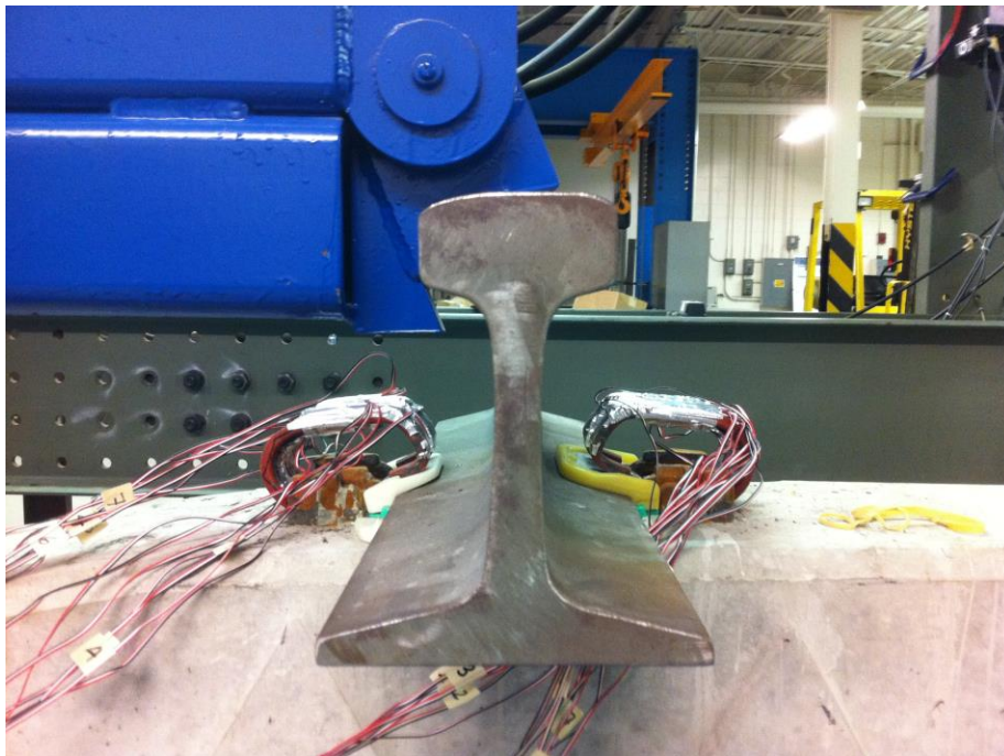
Figure 5.12 Instrumented Clips Used in SLTM Experimentation
