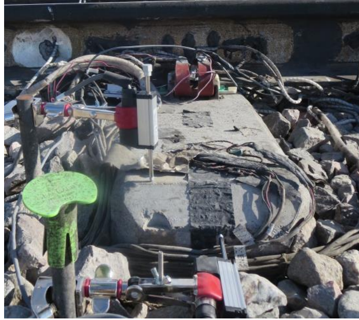
Figure 3.18 Global Crosstie Displacement Measured by Potentiometers Mounted on Rods
