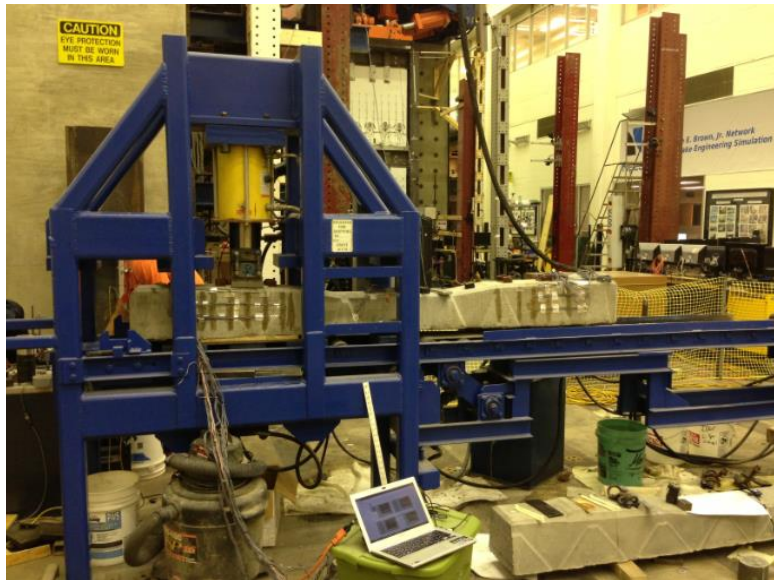
Figure 6.1 Vertical Rail Seat Loading Applied by STT
