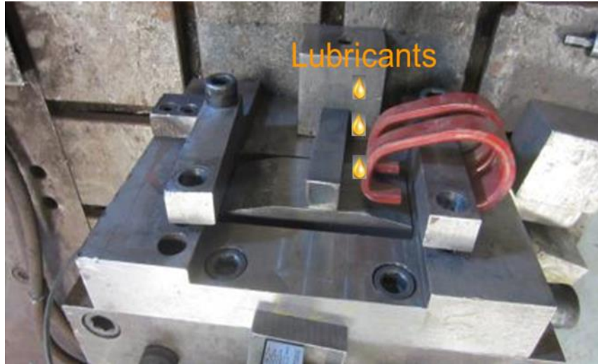
Figure 5.3 Standard Clip Test Required by AREMA (2012)
