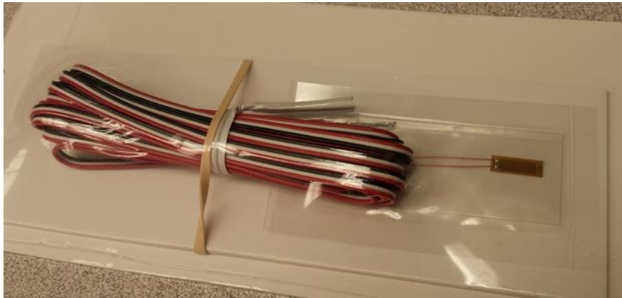
Figure 3.9 Standard 120-ohm Foil Type Shear Strain Gauge
