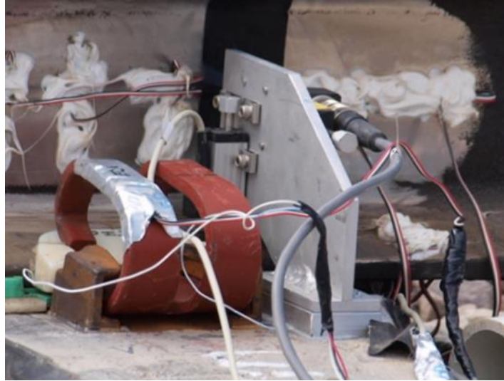
Figure 3.19 Aluminum Fixture for Potentiometer Placement
