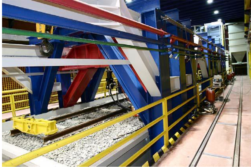
Figure 2.11 Track Box During Testing (NGI 2005)
