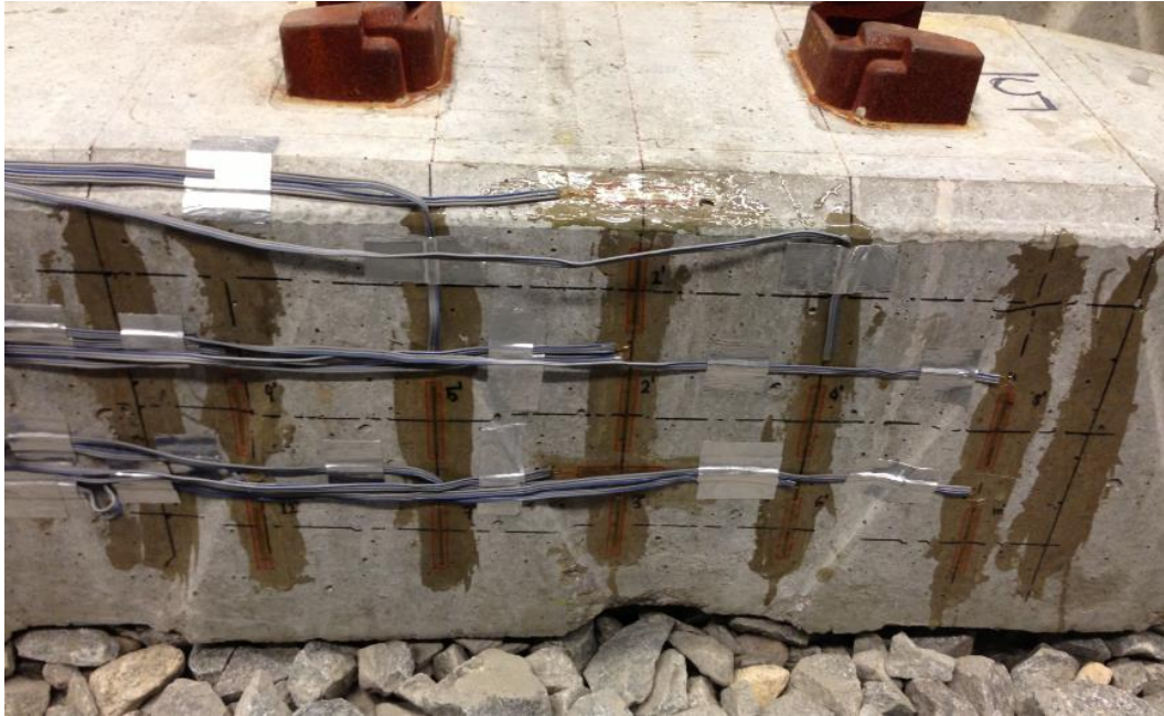
Figure 3.15 External Crosstie Strains
