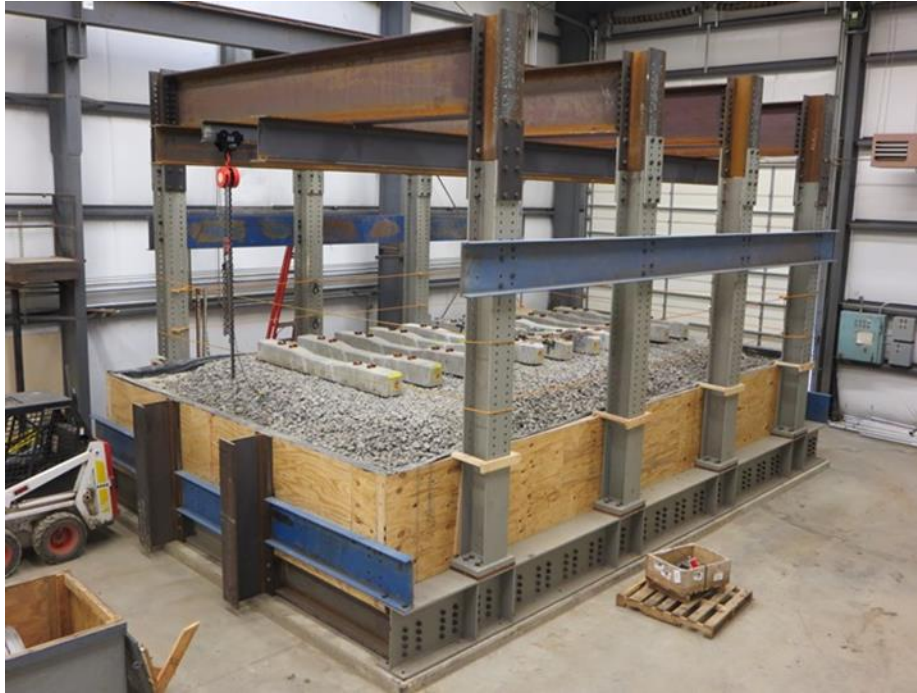
Figure 3.6 Full-Scale Track Loading System (TLS)
