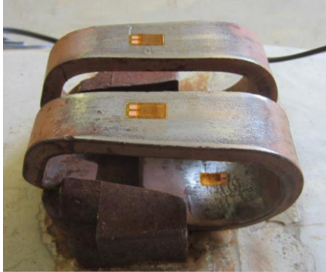
Figure 3.16 Strain Gauges on Clip
