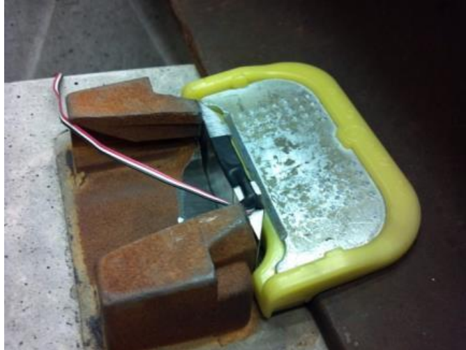
Figure 3.17 Strain Gauges Installed on Shoulder Prior to Clip Application
