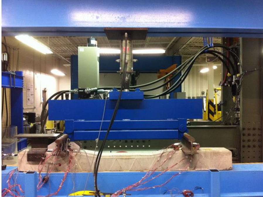
Figure 3.2 Static Load Testing Machine (SLTM)
