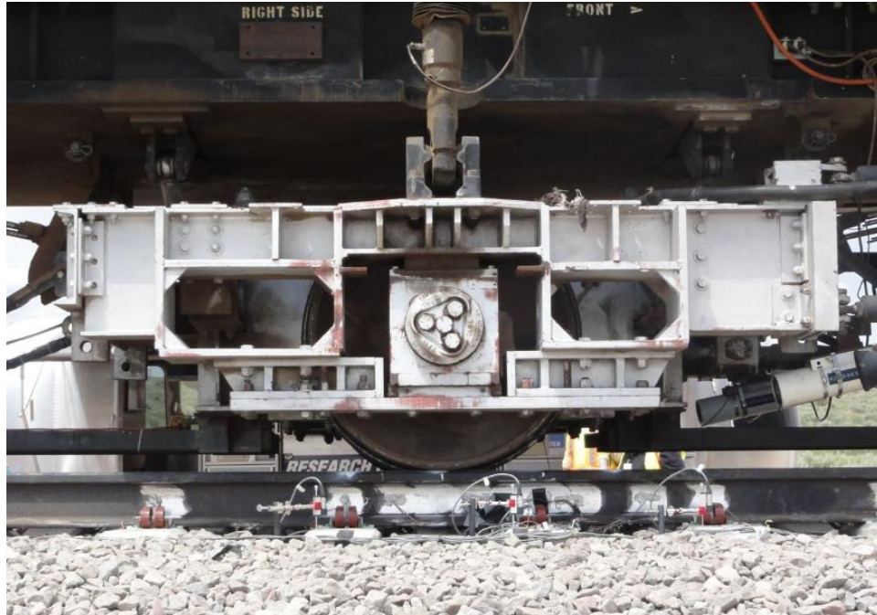
Figure 4.43 Vertical Wheel Load Applied by Hydraulic Actuators
