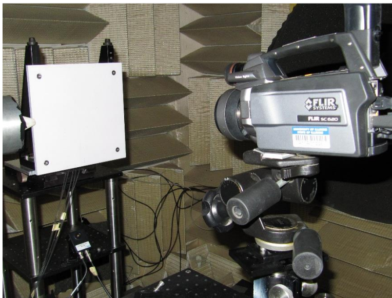
Figure 123. The infrared camera experimental setup for rigid-surface model temperature measurements.
