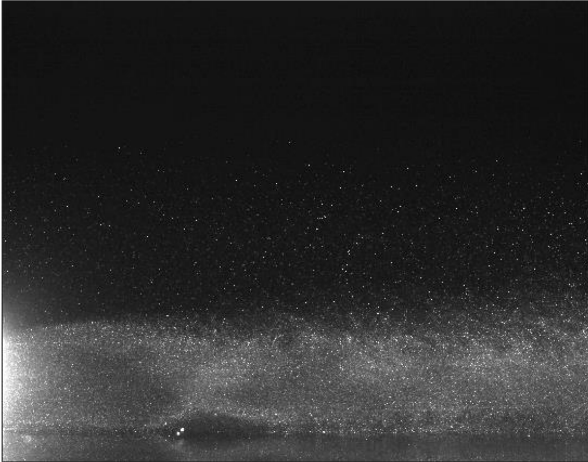
Figure 14. A representative PIV particle image near the nozzle exit.
